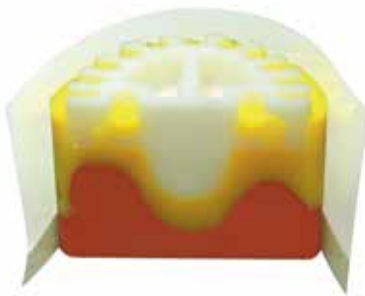
Cross-section of a flaskless duplicating mould
